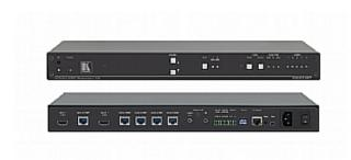
The VM-214DT is a 4K UHD looping distribution amplifier for HDMI & HDBaseT signals. It reclocks and equalizes the signal and distributes it to four identical HDBaseT outputs and a looping HDMI output. It supports resolutions up to 4K@60Hz (4:2:0) UHD. This product offers the versatility of control options and audio de-embedding.
