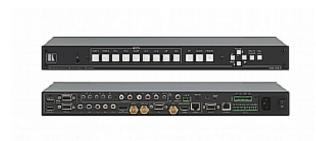
The VP-771 is a high-quality presentation switcher and scaler for a variety of signals. It accepts one of nine inputs: component video, DisplayPort (DP), 3G HD-SDI, two computer graphics, two composite video and two HDMI signals. It scales the video, embeds the audio, and outputs the signal to one HDMI, one computer graphics, one 3G HD-SDI and one DGKat TP, together with digital audio, unbalanced stereo and a 2x10-watt amplified balanced stereo speaker output.
