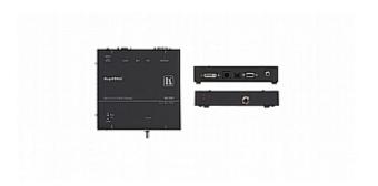
The VP-791 is a high-performance digital scaler for 3G HD-SDI signals. It up- or down-scales the incoming signal, processes the image with HQV and flexible geometry correction and outputs the signal to a DVI/HDMI connector.
