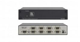
The VP-8K is a highperformance distribution amplifier for computer graphics video signals with resolutions up to and exceeding UXGA. It takes one input, provides correct buffering and isolation, and distributes the signal to eight identical outputs.
