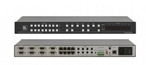
The VP-8x8TP is a high-performance matrix switcher for computer graphics video and stereo audio signals. The unit routes any or all inputs to any or all twisted pair outputs. A compatible twisted pair receiver converts each output signal back to the original input formats.
