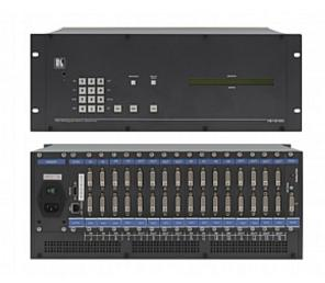
The VS-1616D is a high-performance matrix switcher chassis for DVI & HDMI signals. The unit is modular and populated from 2x2 to 16x16 in increments of two inputs and/or two outputs. The chassis includes a power supply, control module and a test module that can monitor and test any input and output in the matrix.
