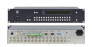
The VS-1616SDI is a high-performance matrix switcher for SDI (SMPTE 259M) video signals. Switching is implemented during the vertical interval period according to the SMPTE RP-168 standard, when using synchronized SDI sources.
