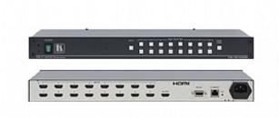
The VS-161H is a highperformance switcher for HDMI signals. It reclocks and equalizes the signal and switches one of the 16 inputs to a single HDMI output.
