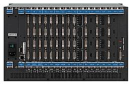
The VS-3232DN is a high-performance matrix switcher chassis for DVI & HDMI signals. The unit is modular and populated from 4x4 to 32x32 in increments of four inputs and/or four outputs. The chassis includes one power supply but can also accept a second redundant power supply (sold separately), a control module and a test module that monitors and tests any input and output in the matrix.
