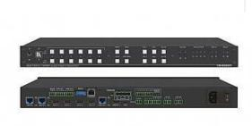
VS-622DT is an all-in-one 4K@60Hz (4:2:0) presentation system with 6x2 HDMI/HDBaseT matrix switching, control gateway, PoE, power amplifier, and Maestro room automation. The unit reclocks and equalizes the signals and can route any input to the HDMI or the HDBaseT output or to both outputs simultaneously. It supports resolutions up to 4K@60Hz (4:2:0) and WUXGA.
