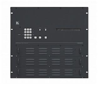
The VS-6464DN is a high-performance matrix switcher chassis for DVI & HDMI signals. The unit is modular and populated from 8x8 to 64x64 in increments of eight inputs and/or eight outputs. The chassis includes a power supply, control module and a test module that can monitor and test any input and output in the matrix.
