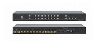
The Kramer VS-82HDxl is a true 8 x 2 matrix switcher for SDI signals. The unit can switch any one of the eight SDI inputs to one or both sets of triple outputs (two-channel SDI and HDMI).
