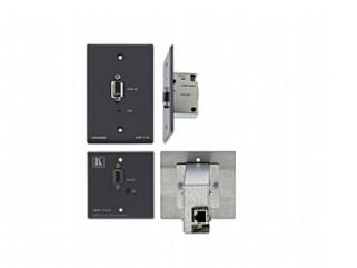
The WP-110 is a wall plate twisted pair transmitter for computer graphics video signals with resolutions up to and exceeding UXGA. It converts a computer graphics video signal into a twisted pair signal that the TP-120 twisted pair receiver (or other compatible Kramer receiver) converts back into a computer graphic signal.
