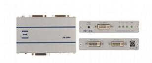
The XE-12D is a compact, high-performance distributor for DVI-D signals. The device takes one input and distributes the signal to two identical outputs on DVI connectors.
