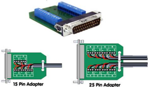
Adapter PCBs which can be used on LYNX modules with SubD connections allowing the direct connection of cables using the terminal blocks provided. A convininet alternative to manually soldering SubD connectors or using one of the available adapter cables. Intended for use with Series 5000 modules in a permanent system environment.
