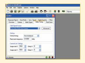
Included with MIL is the Matrox Intellicam frame grabber configuration utility<sup>3</sup>.
