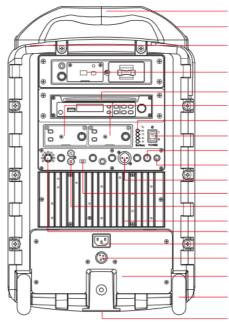
Molded Fixed Handle Retractable Carry Handle Transmitters Storage for 2 transmitters Optional MRM-72 or MTM-90 Optional CDM-2 CD Player Optional 2 MRM-70 Receivers 4-segment Battery Level Meter Power Switch Echo Control on wireless mics Extension Speaker Output Mic Inputs: XLR & 6.3mm (1/4") Voice over Music Priority Switch RCA Line-input/output Jacks Heat Sink Digital Master Volume AC Switching Power Input Socket 24~32V DC Input Jack **Built-in Rechargeable Batteries** Trolley Wheels
