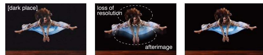
Without Noise Reduction Some noise is evident when gain control is turned up 3D Noise Reduction Alone Afterimage and some loss of resolution is seen New Hybrid Digital Noise Reduction Clearer images in difficult conditions
