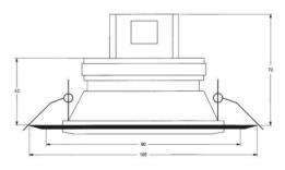
The hole cutout required for mounting should have a diameter of 90 mm +/- 3 mm.
