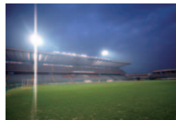
Conventional CCD Sensor (vertical smear)
