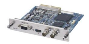
The HFBK-HD1 is an HD SDI Output Board for the HFU-X310 Optical Interface Unit which is used with the HDC-X310/X310K HD multi-purpose camera.
