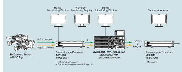
Fig 1 3D production System Configuration Example
