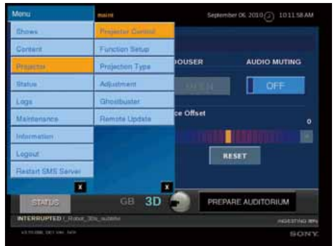
Menu window of LKRA-003 Touch Panel Monitor (projectionist terminal)
