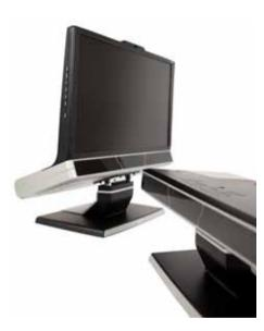
The Tobii TX300 Eye Tracker sets a new standard for remote eye trackers. Its unique combination of 300 Hz sampling rate, very high precision and accuracy, robust tracking and compensation for large head movements extends the possibilities for unobtrusive research of oculomotor functions and human behavior.
