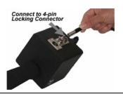
3. Connect the <u>4-pin XLR power cable from the AC adapter to the 4-pin XLR power connector located on the MC100 Control Unit.</u>
