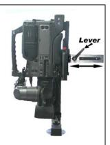
5. Engage the brass motor gears to the black arm gears and tighten. Be sure the levers are pointing <u>away</u> from the rotating arm. -NOTE: Once tightened, you can adjust the position of the lever by simply pulling out on it and then rotating the lever until it faces away. This will NOT loosen the fastener. Failure to aim lever away will impede the movement of the MC100.
