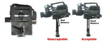
(you may want to use multiple bolts for large cameras with tripod mounting plates).
