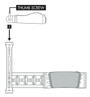
Loosen THUMB SCREWS to adjust HANDLES to desired position
