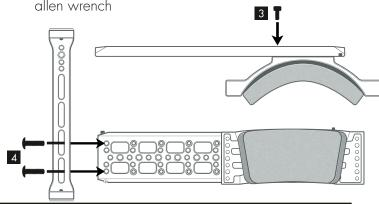
Select HANDLES, attach to CROSSBAR using THUMB SCREWS
