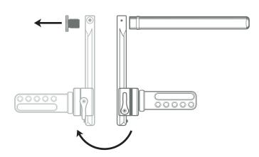
NOTE: To change viewfinder position, remove ROD END CAP, flip NATO RAIL, reinstall and adjust viewfinder using KNUCKLE THUMBSCREW
