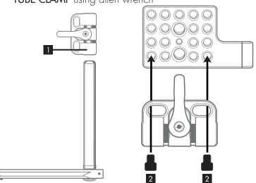
3. Slide NATO RAIL KIT into TUBE CLAMP, tighten using THUMB SCREW
