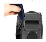
2 Use T9 Torx wrench to remove (4) screws from top of camera.
