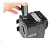
Install (4) M4 button head screws in corresponding holes.
