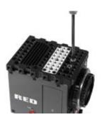
Install (2) 1/4-20 socket cap screws in corresponding holes.
