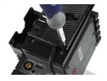
Align battery plate on Fixed Back.
